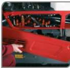
Under seat component access- the battery and electrical components are conveniently located under the operator seat. 12 volt power sockets with two on cab model.
